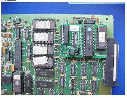
Locate and remove the Z80 chip on the CPU board. Use the photos to assist in locating it.
