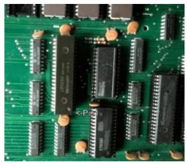
2. Install the z80 onto the daughter card then attach on PCB like this. [Ensure PIN 1 of the z80 is installed with the proper orientation]-
