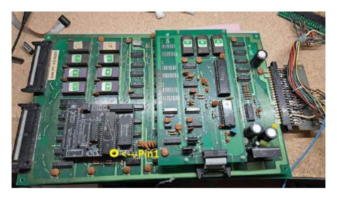
Verify that the kit is seated fully in the socket and nothing is touching the underside -
