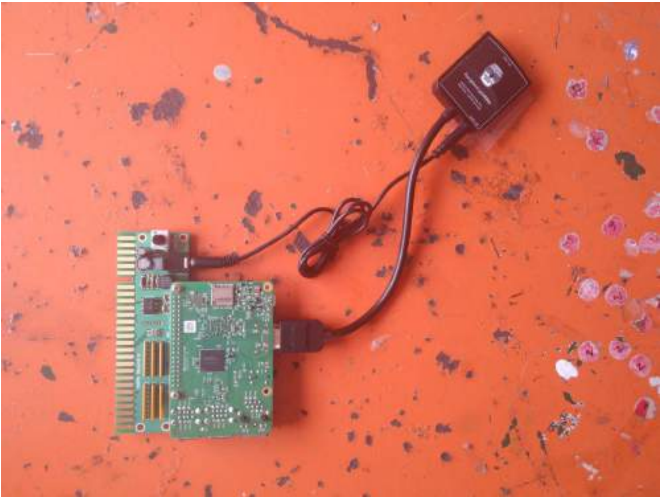
RaspberryJAMMA mini with RPi3B+, setup for use with VGA video output, 3.5mm audio links DAC audio output to RaspberryJAMMA mini audio input.
